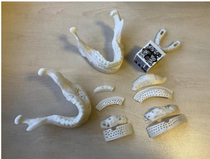
Figure 2: Biomodels and surgical guides. Surgical guide integrated with a QR code.
